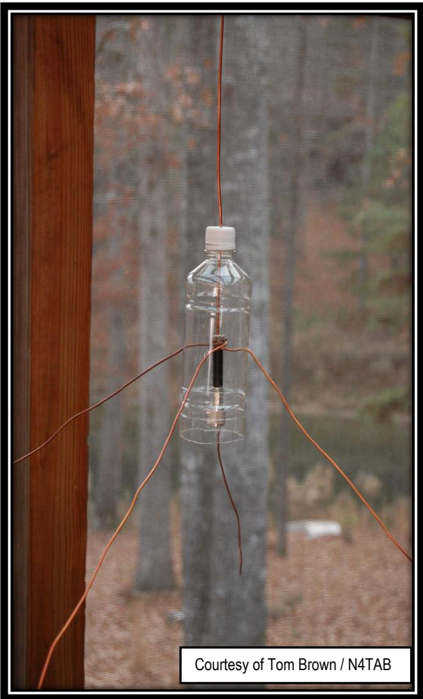
Figure 2. Example of VHF Ground Plane Antenna
