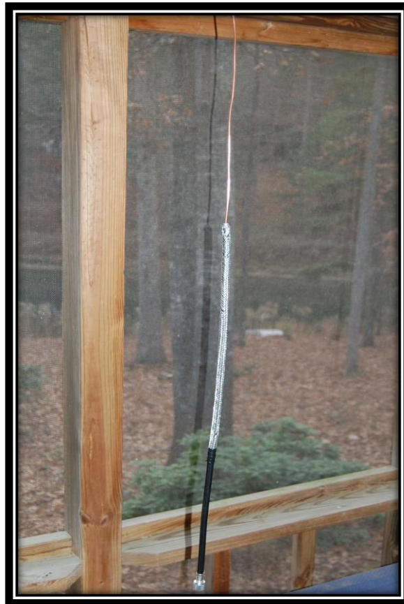
Figure 4. Example of VHF Coaxial Sleeve Antenna
